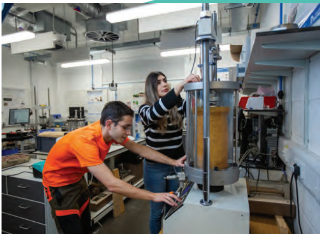
PhD students Rafael Periera-Anjos and Saba Ghassemi performing cyclical triaxial testing of scaled railway ballast with novel geosynthetic reinforcements
